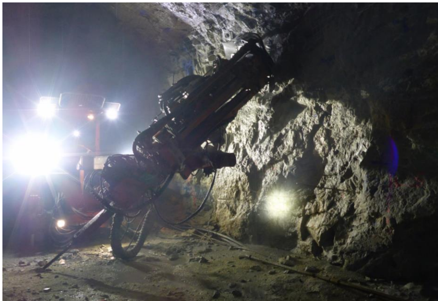
Figure 7. Long Hole Rig drilling the 1394 Long Hole Stope between 1394 to 1410 Levels.
