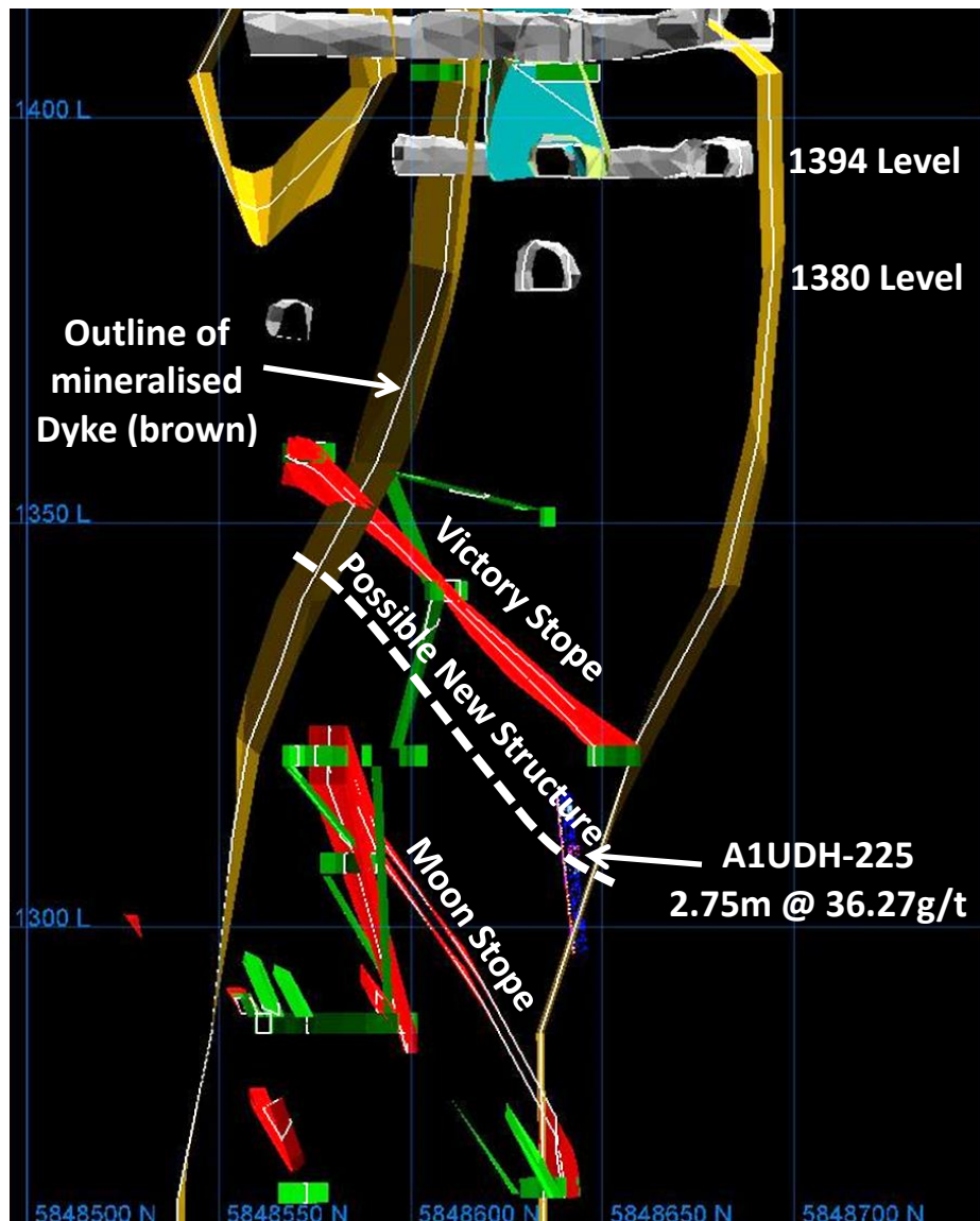
Figure14. Cross Section of the A1 Dyke (outline shown in brown) showing the present working levels, historical development (green) and stoping (red) with location of A1UDH-225.
