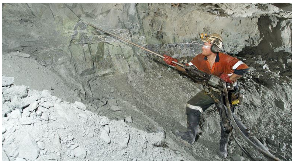
Figure 3. Photograph of air leg miner, Nathan Hicks, drilling holes at the 14 Level 840 Stope at the A1 Gold Mine.
