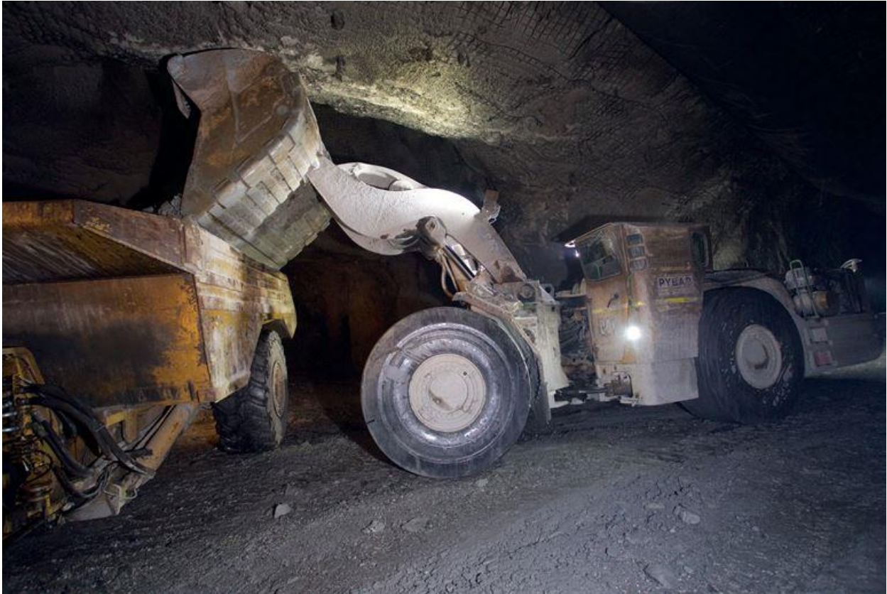
Figure 6. The 1700 LHD loading an underground truck at the 1410 Level of the A1 Gold Mine.
