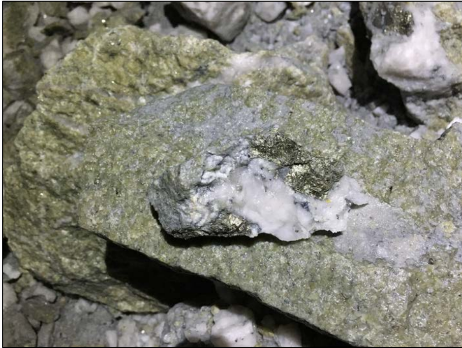
Figure 4 and 5. Photographs of heavily veined and strongly altered High Grade Ore in development. Taken at the intersection of the 1394 Ore Decline with the Indicated Resources (shown in Magenta in Figure 3, above).
