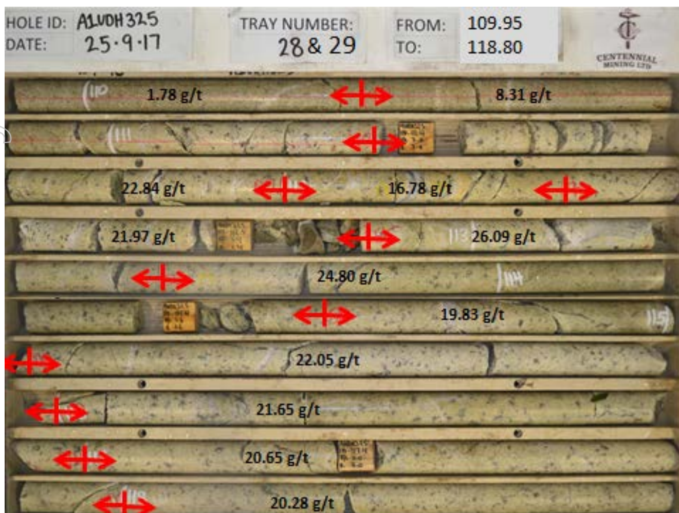
Figure 4: Queen's exploration target diamond drill core from A1UDH-325 showing grades against Lithology
