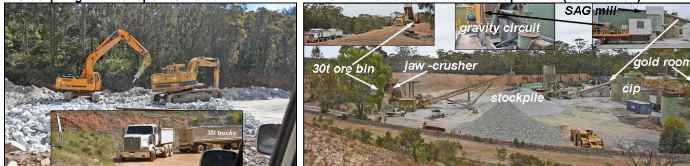
Figure 12. Stockpiling and Transport to Maldon, View of the Maldon Plant at Porcupine Flat (near Maldon) a. Stockpiling and Transport to Maldon b. View of the Maldon Plant at Porcupine Flat (near Maldon)
