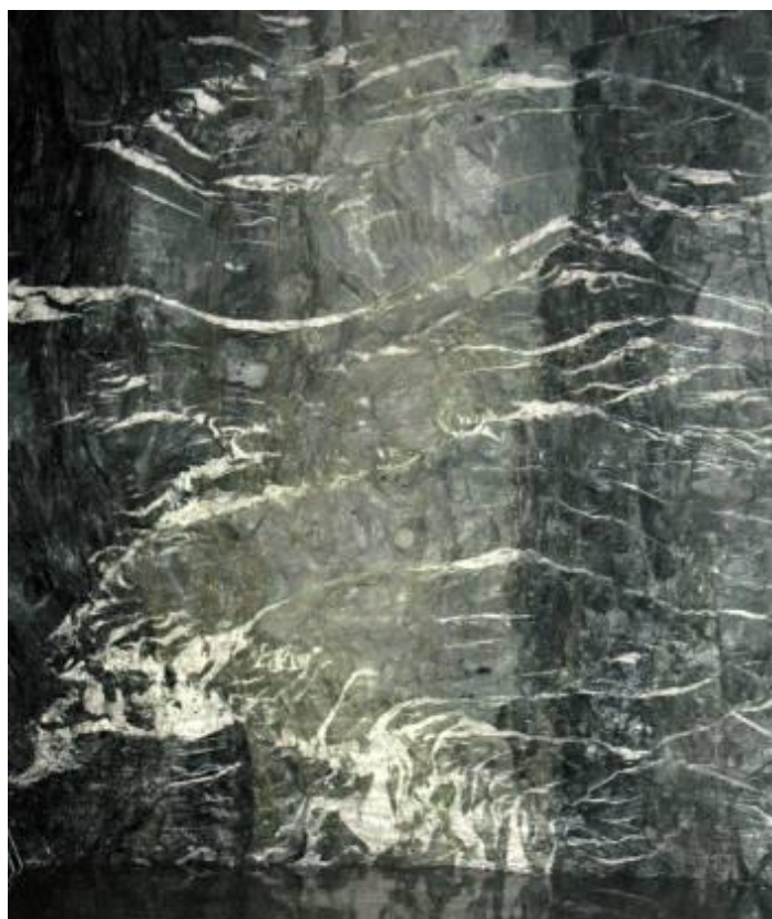
Figure 3-3: Ladder veins tending to stockworks at the 7 Level, A1 Mine. The dyke is the paler rock at the centre and right of the photo. Dark grey rocks are sediments. Note the stockwork development towards the bottom left-hand corner where a reverse fault has thrust the dyke over the sediments. Face is approximately 2m across.
